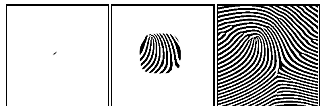
Fig. 7. Intermediate ridge patterns generated using Gabor filtering. The number of iterations increases from left to right.
